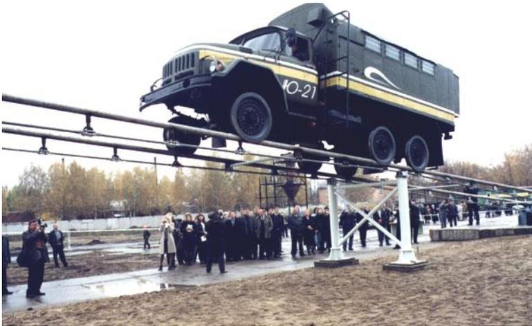
**Fig. 1. UST in the town of Ozyory, Moscow Region, October 2001. Module simulator – modified automobile ZIL-131 with the total weight of 12 tons**
