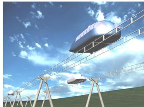
**Fig. 4. High-speed module, travel speed – up to 400 km/hour, carrying capacity – 30...60 passengers**
