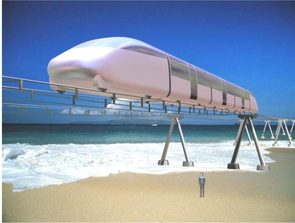
**Fig. 7. Passenger UST train, travel speed up to 350 km/hour, carrying capacity – up to 500 passengers**
