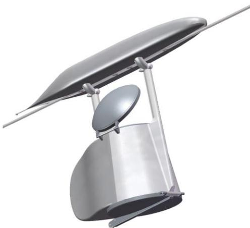
Figure 7: Unicar with loading hatch opened
