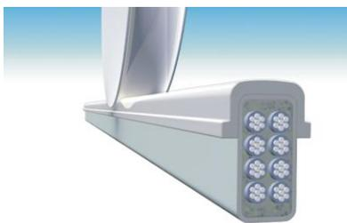
Fig. 5. Design of a string-rail and a wheel
